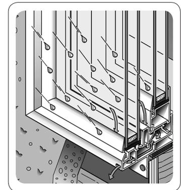
Once a year before the rainy season, check the sill to ensure that the sill remains clean. Vacuum to remove debris in the sill. Check the sill for good sealant adhesion. Some locations on the window to check would be the jamb corners at the head and sill or the joints between the center post and the head and sill. If necessary, re-seal these joints with an acrylic small joint sealant. This sealant is available at a local window store.
