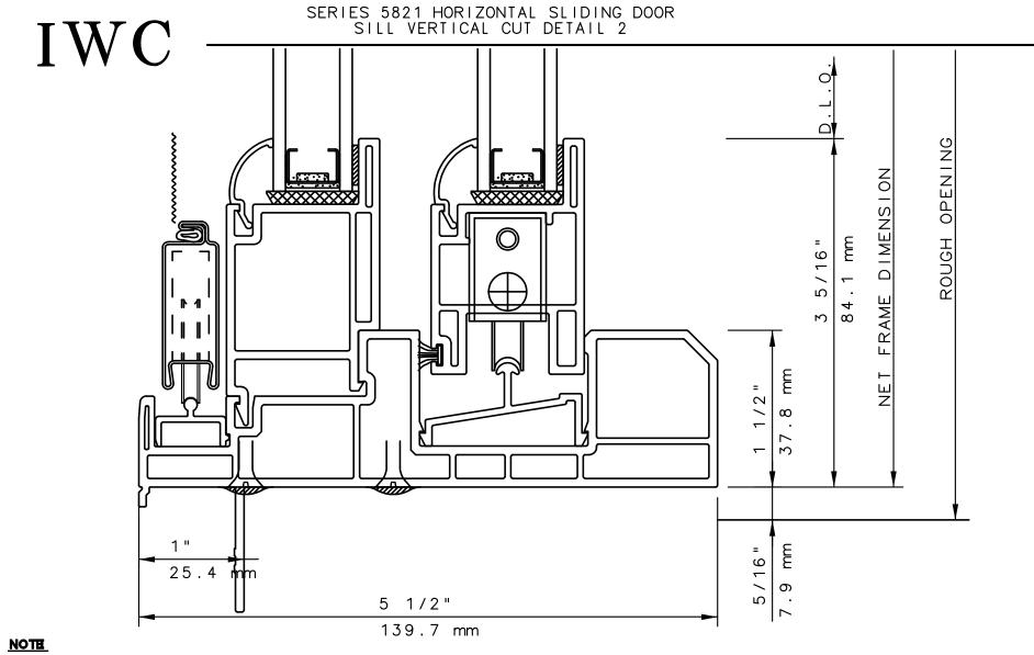
THIS IS AN ARCHITECTURAL VIEW OF CROSS SECTIONS ONLY AND INSTALLATION OF SHIMS, FASTENERS, AND SEALANT SHALL BE THE RESPONSIBILITY OF THE INSTALLER.
