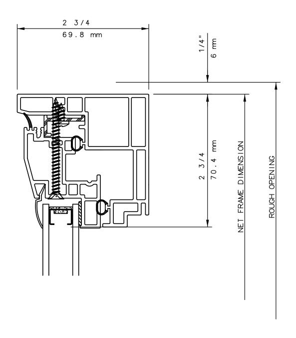
THIS IS AN ARCHITECTURAL VIEW OF CROSS SECTIONS ONLY AND INSTALLATION OF SHIMS, FASTENERS, AND SEALANT SHALL BE THE RESPONSIBILITY OF THE INSTALLER.
