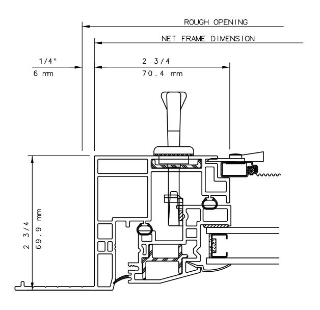
THIS IS AN ARCHITECTURAL VIEW OF CROSS SECTIONS ONLY AND INSTALLATION OF SHIMS, FASTENERS, AND SEALANT SHALL BE THE RESPONSIBILITY OF THE INSTALLER.
