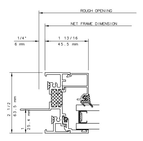
THIS IS AN ARCHITECTURAL VIEW OF CROSS SECTIONS ONLY AND INSTALLATION OF SHIMS, FASTENERS, AND SEALANT SHALL BE THE RESPONSIBILITY OF THE INSTALLER.
